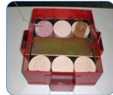
Example of solid aerosol-forming condensed aerosol material
